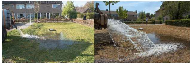
Figure 9.42 Swale at Dalfsen (the Netherlands) showing normal condition on the left in 2017 and on the right the same swale after a 7 week dry period in 2018. Source: Boogaard (2022).
